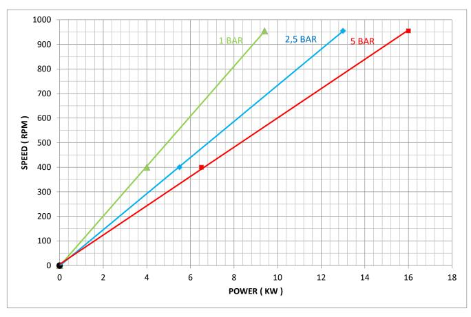
TESTS HAVE BEEN DONE WITH SAE30 OIL AT ROOM TEMPERATURE (APPROX. 100 CST)
